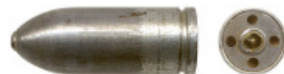
Fig. 29-8. 13mm Zinc (or tin)-plated presentation Gyrojet dummy with exposed primer anvil, 12.9 x 35.8mm..
