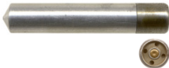
Fig. 29-10. 13mm Dummy "flare" with metal pieces inside, 12.9 x 70.8 mm.
