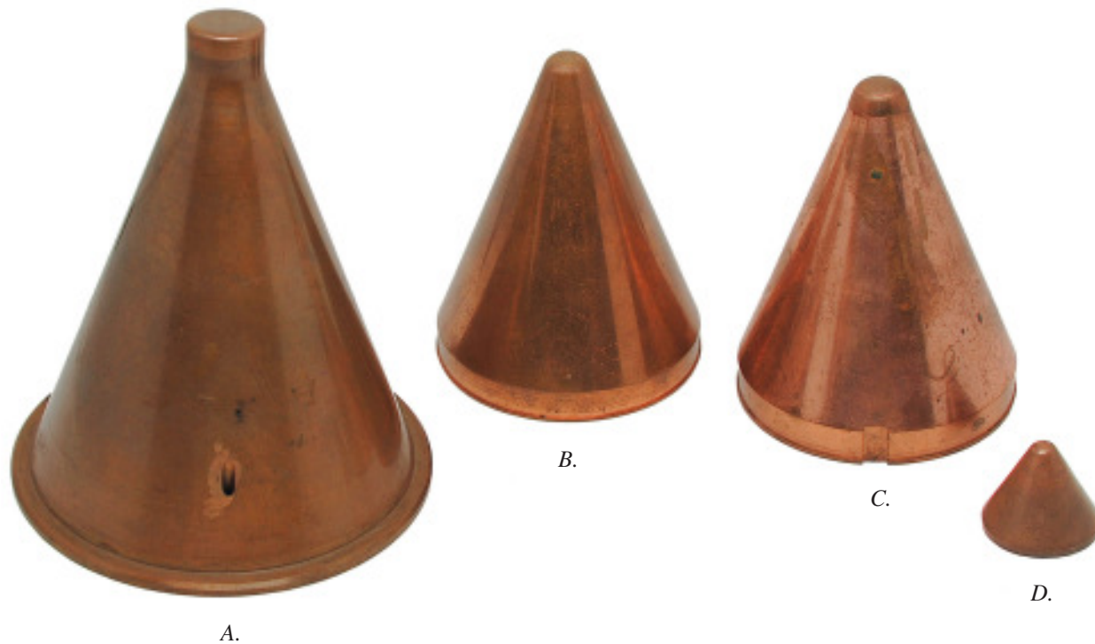
Fig. 29-22. Solid copper high explosive shaped charge liners made by MBA. (A.) 95.3mm diameter at large end, including flange. (B.) 66mm diameter. (C.) 66mm diameter. (D.) 25.2mm diameter.
