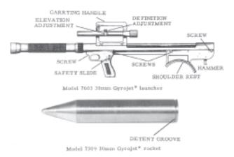
Fig. 28–87. MBA 30mm Model 7309 rocket and Model 7603 weapon system. MBA drawing and photo.
