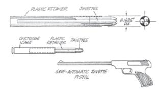
Fig. 28–26. Experimental .25-caliber Javette-launching cartridge.
