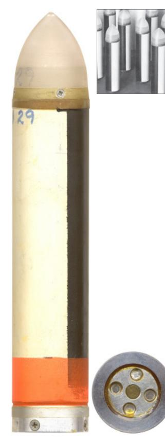
Fig. 28–95. 40mm Type I cloud seeding rocket and MBA photo.
