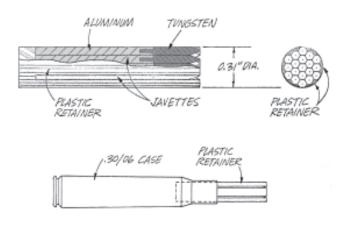
Fig. 28-25. Experimental .30-06 Javette-launching cartridge.
