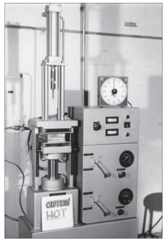
*Fig.* 28–38. *MBA Methocel Javette heat mold, closed, heat applied. MBA photo.*
