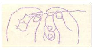
Carefully place the small square of onion skin paper [?] onto the Microjet; press the paper toward the tail so that the fins are halfway inserted. This acts as a hold down, allowing the rocket to build up to full thrust before leaving tube.
