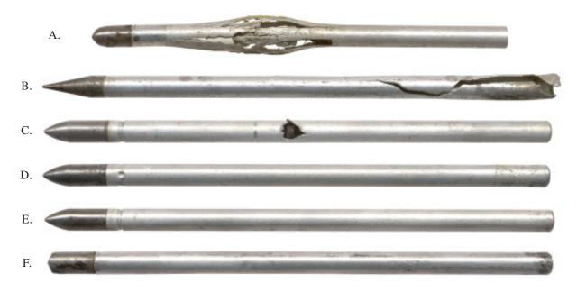
Fig. 28–23. .25-caliber experimental anti-mine Lancejets, actual size. (A) Premature PETN detonation at delay train. Propellant grain mostly intact. (B) Case failure at motor section. (C) Case failure at delay train position. (D) Point with stab crimps. (E) Point with heavy cannelure. (F) Blunt nose point with no crimp.
