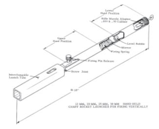
Fig. 28-80. Multi-caliber Gyrojet flare launcher. MBA drawing.
