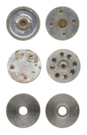
Fig. 28–58. MBA 30mm steel rocket nozzles. Actual size.
