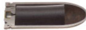
Fig. 6-12. Nickel-plated 13mm Gyrojet dummy section with rubber “grain.” Note the empty nickel-plated primer cup. Actual size.
