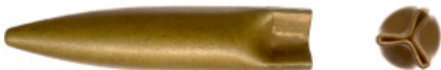
Fig. 6–5. Pinched-base .50-caliber (12.87 x 58.08mm) Gyrojet and its nozzle. This Gyrojet has a small remnant of BKNO_3 -coated copper wire fuse in the center of its nozzle. Actual size.
