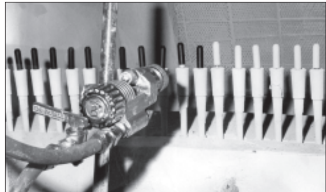
Fig. 6–15. Applying titanium oxide in spray booth. MBA photo.
