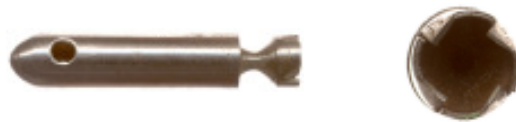
Fig. 6–6. .30-caliber (7.62 x 38.4mm) Gyrojet with fluted-vane nozzle, actual size. Nozzle shown 2x actual size. Key-chain dummy souvenir. Woodin Laboratory.
