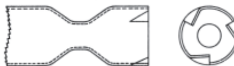
Fig. 27–17. MBA proposed anti-mine Lancejet nozzle. USAERDL Report 1828.
