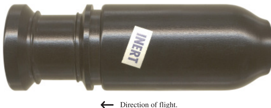
Figure 27-58. 40mm MBA dummy ARROW multiflechette rocket variation, actual size..
