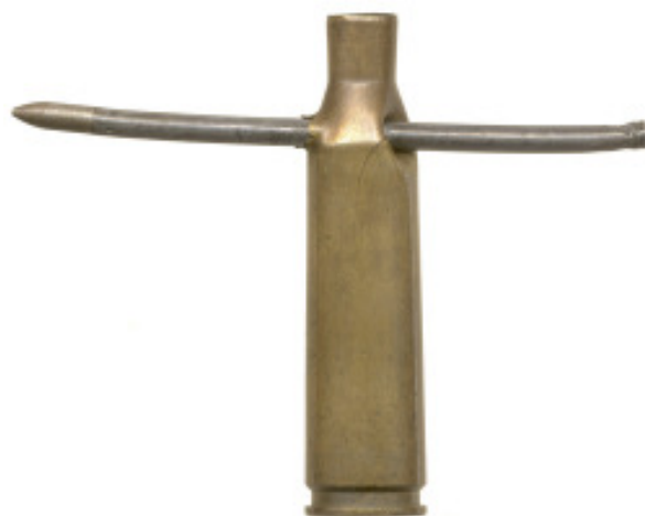
Fig. 27–20. MBA .25-caliber anti-mine Lancejet in a fired .60-caliber cartridge case.
