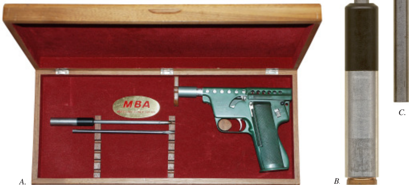
Figure 27–36. 13mm Survival pistol, serial number B5113S (A); Spear round (B), actual size; and spear variation (C), actual size.
