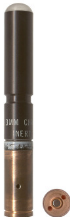
Figure 27–39. MBA 13mm dummy chaff flare with one hole in the motor section. Actual size.
