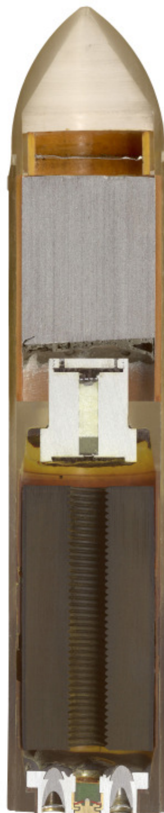
Figure 27–50. 40mm cloud-seeding rocket section.
